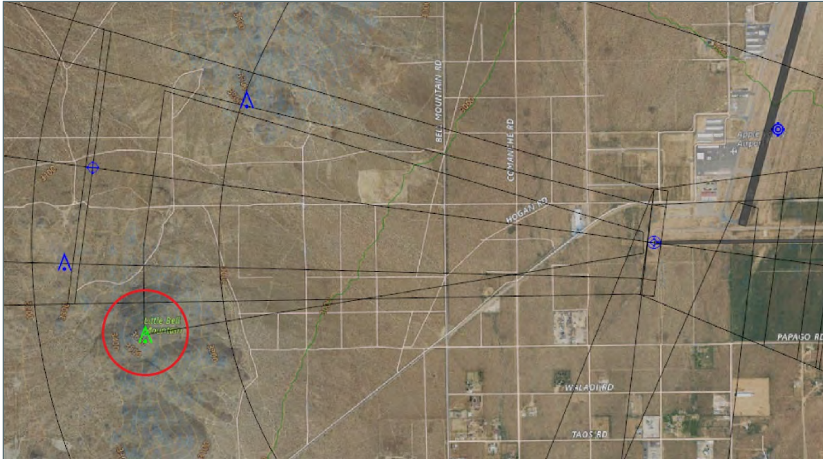
Figure 5-1: TERPS Penetration Preventing Nighttime Operations to Runway 8-26
